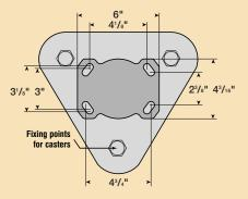
When fitting at 4-3/4" x 2-3/8" hole centers, use 1/2" diameter bolts. When fitting at 4-1/8" x 3-1/8" hole centers, use 1/2" diameter bolts.
